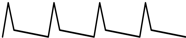
FIGURE 11. VOLTAGE ACROSS R WITHOUT RC
