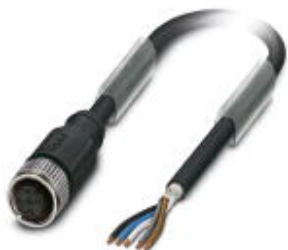
Sensor/actuator cable, 5-position, PUR/PVC, gray RAL 7001, shielded, free cable end, on Socket straight M12, A-coded, cable length: 10 m, Tin-plated wire ends, with shrink sleeves
