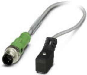
Sensor/actuator cable, 2-pos, PUR/PVC gray, straight M12 plug on valve connector type MSZC, with 1 LED, cable length: 2.5 m
