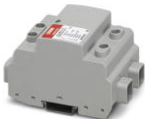
Lightning/surge arrester for 2-pos. isolated 1500 V DC voltage systems, for DIN rail mounting, temperature-monitored protective elements, status message on the module.
