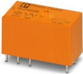
Plug-in miniature power relay in basic design, with power contact, 2 PDTs, input voltage 24 V DC
