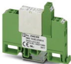
Relay module, with soldered-in miniature switching relay, gold contact for small loads, 1 PDT, input voltage 24 V DC, design rotated by 180°
