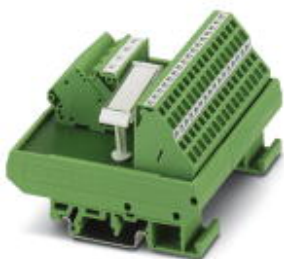
VARIOFACE module, with two equipotential busbars (P1, P2) for potential distribution, for mounting on NS 35/7.5 or NS 32. Module width: 90 mm
