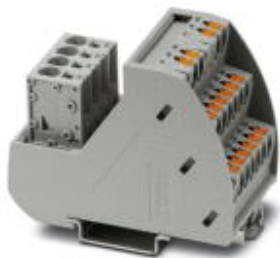
VARIOFACE module, with two equipotential busbars (P1, P2) for potential distribution, for mounting on NS 35 rails. Module width: 41.9 mm
