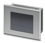
Touch panel with 9.7 cm/3.8" FSTN-display (analog resistive (polyester)), 320 x 240 pixel(s) (QVGA), 5 grayscales, Arm9<sup>™</sup>, 200 MHz, 2x USB host 2.0, 1 x Ethernet (10/100 Mbps), RJ45, Windows CE 5.0 and user software: TSvisRT. (bus system: without)
