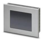
Touch panel with 8,9 cm / 3,5"-TFT-display (analog resistive (polyester)), 320 x 240 pixel(s) (QVGA), 65536 colors, Arm9 $^{\text{TM}}$ , 200 MHz, 2x USB host 2.0, 1 x Ethernet (10/100 Mbps), RJ45, Windows CE 5.0 and user software: TSvisRT / TSDiag. (bus system: without)
