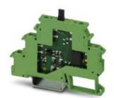
Input solid-state relay terminal block, input: 24 V DC, output: 3 - 48 V DC/100 mA, with isolating plug in output, terminal block width: 6.2 mm
