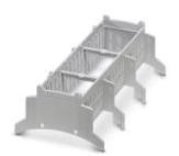
DIN rail housing for use in distribution boards in accordance with DIN 43880, Upper housing part with vents, Installation depth connection technology: 22.35 mm, width: 161.6 mm, height: 89.7 mm, Depth: 54.85 mm, color: light gray (7035)
