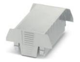
DIN rail housing, Upper part, connection opening on both sides, width: 90.1 mm, height: 74.65 mm, Depth: 36.95 mm, color: light gray (7035)
