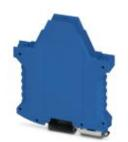
DIN rail housing, Lower housing part with metal foot catch, tall design, with vents, width: 17.6 mm, height: 99 mm, Depth: 107.3 mm, cross connection: DIN rail bus connector, number of positions cross connector: 5, color: blue (5015)
