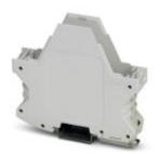
DIN rail housing, Lower housing part with metal foot catch, flat design, without vents, width: 22.6 mm, height: 99 mm, Depth: 84.8 mm, cross connection: DIN rail connector (optional), number of positions cross connector: 5, color: light gray (7035)
