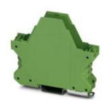
DIN rail housing, Lower housing part with metal foot catch, flat design, without vents, width: 22.6 mm, height: 99 mm, Depth: 84.8 mm, cross connection: without bus connector, number of positions cross connector: not relevant, color: green (6021)
