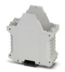
DIN rail housing, Lower housing part with metal foot catch, tall design, with vents, width: 45.2 mm, height: 99 mm, depth: 107.3 mm, cross connection: DIN rail connector (optional), number of positions cross connector: 5, color: light gray (7035)
