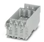
DIN rail housing, Lower housing part with metal foot catch, with vents, width: 75.9 mm, height: 120.6 mm, depth: 64.3 mm, cross connection: DIN rail connector (optional), number of positions cross connector: 8, color: light gray (7035)
