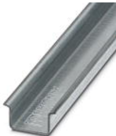
DIN rail, unperforated, Standard profile, width: 35 mm, height: 15 mm, similar to EN 60715, material: Steel, galvanized, length: 3000 mm
