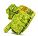
Pick-off terminal block, For use with PTPOWER 50, 95, 150, and 185 Power-Turn high-current terminal blocks, nom. voltage: 1500 V, nominal current: 57 A, connection method: Push-in connection, number of connections: 2, cross section: 0.5 mm² - 16 mm², AWG: 20 - 6, width: 18.5 mm, height: 34.7 mm, color: green/yellow, mounting type: on base element
