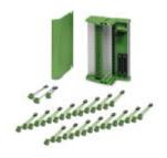
Termination Carrier for redundantly connecting 16 MACX Analog Ex i signal conditioners to analog input cards of the Yokogawa CENTUM VP controller, via two KS40 connectors, 40-pos. Suitable for Yokogawa AAI141 and AAI143 cards.
