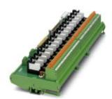
16-channel relay module for Honeywell C300 input modules. The module is controlled by the control system via 37-pos. D-SUB or 50-pos. FLK. A screw connection with knife disconnection is available in the field. Module width: 343 mm
