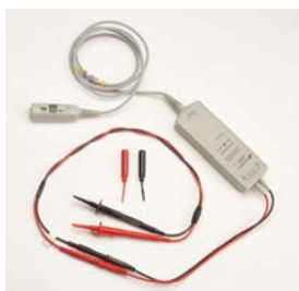
N2790A high voltage differential probe with N7013A extreme temperature extension kit
