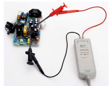
N2790A measuring a power supply signal
