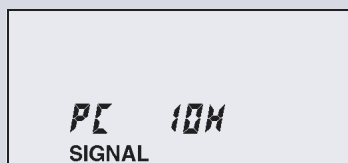
Figure 4. 10 Base-T signal detected, wired to PC.
