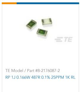
Surface Mount Resistors, Precision Resistor, 2 Terminations, Size Code 0603, Taped & Reeled, .1%, Thin Film, Resistance Range Up to  $1k\Omega$   $\Omega$
