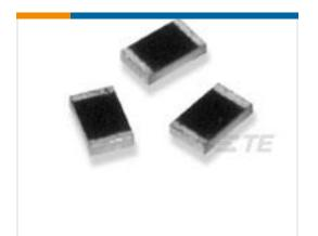
TE Model / Part # 9-1879252-4 RP 2B 10R 0.1% 15PPM CUT LENGTH
