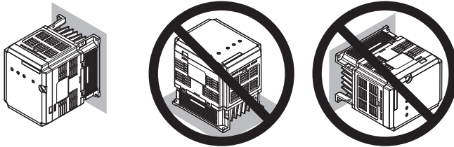
Figure 8 Correct Installation Orientation (Braking Unit)
