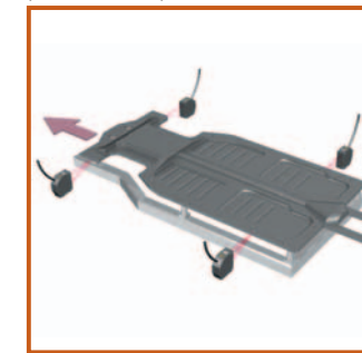
Measuring Car Body Widths (ZS-HLDS10)
