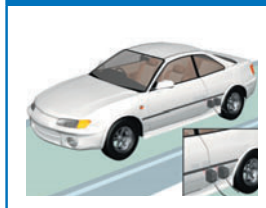
Measuring Door Attachment Offsets
