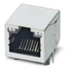
RJ45 socket insert, type: RJ45, degree of protection: IP20, number of positions: 8, 10 Gbps, connection method: Solder connection
