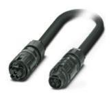
Circular connectors (cable-side), Range of articles: PRC, Connecting cable, housing material: PPE, color: black, number of positions: 3, nom. voltage: 690 V AC, rated current: 24 A, Connection method: Screw connection, Type of contact: Socket/pin
