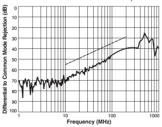
802.3af specification: 45 dB min at 30 MHz 40 dB min at 60 MHz 35 dB min at 100 MHz
