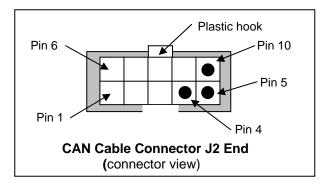
The following table shows the signals present on the CAN cable at the AppBox J2 connector end
