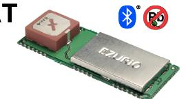
The Ezurio Embedded Bluetooth Module is specifically designed for applications that demand a robust and reliable Bluetooth connection. This product has been designed with solder connections that allow the module to be mounted directly into your own designs and potted or enclosed within a metal housing, while exposing a high performance multilayer ceramic antenna.
