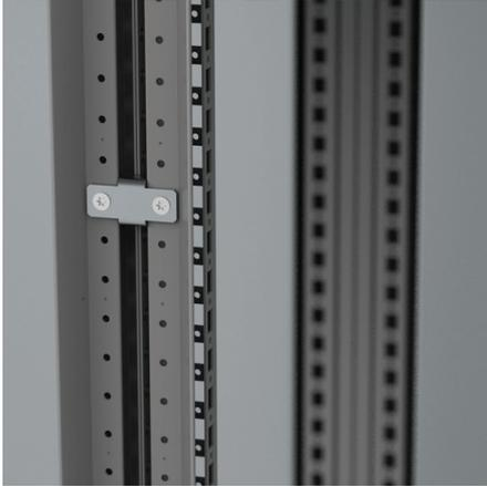
**Description:** Short brackets mounted on the outside hole pattern of the frame of the bayed enclosures with an "auto spacer" function. Specially designed for small doors/panels configuration. This method of baying mild steel enclosures has also the advantage of creating a direct earthing connection between the enclosure frames.
