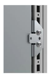
**Description:** For extra fixing of a heavily equipped mounting plate in the far rear position. Mounted directly to the enclosure frame for extra stability. Easy mounting without drilling. Can be fixed from the front even after the mounting plate is already in position. The combination with an MPR profile is advised.
