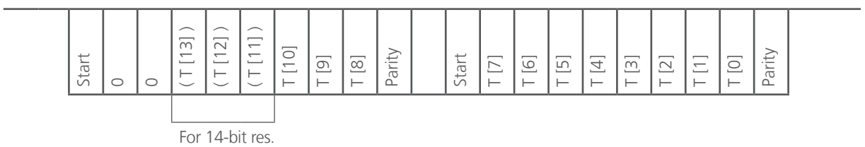
Figure 1.2 – Full ZACwire™ Temperature Transmission from TSic
