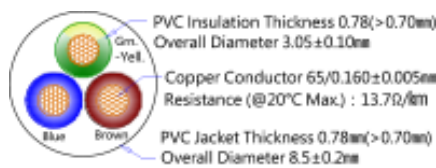
SJT 16AWGx3C (Wire Cross-Section)
