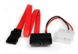
The SLSATAF12 Slimline SATA to SATA with LP4 Power Cable (12-inch) features a SATA data receptacle and a LP4 power connection on one end, and a Slimline Serial ATA receptacle on the other - allowing you to connect a slim SATA drive to a computer motherboard that does not have a Slimline connection available.
