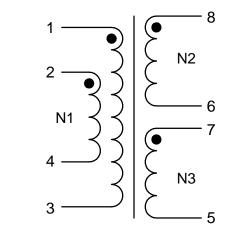
N1 denotes two windings connected in parallel. Terminals 1+2 and 3+4 must be tied as solder bridging is allowed.
