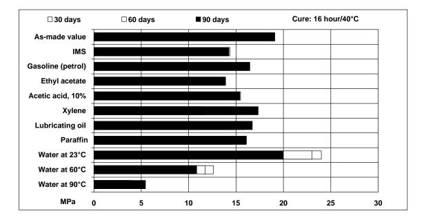
Lap shear strength versus immersion in various media (typical average values)
