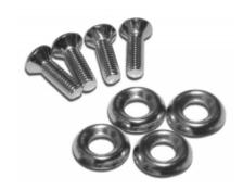
The 1421 screw provides a standard 0.625" rack screws length with 10-32 threads. The screw itself features a slotted oval head and has a nickel plate finish. The steel cup washers have an outside diameter of 0.60".
