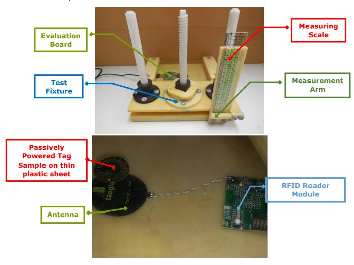
The test sample is placed on a thin sheet of plastic connected to the movable part of the fixture. Then the distance is carefully adjusted until the reader can no longer read the sample, thus the maximum interrogation distance is displayed in the ruler.
