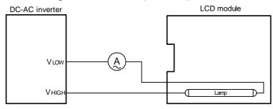
\*Connect the High Frequency Current Meter to the Low-Voltage (VLOW) side.
