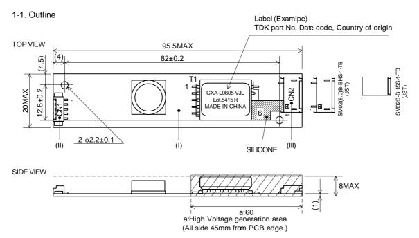
Please secure the air clearance of 2mm or more from the high voltage generation area up and down and right and left. Please refer to Note1-3. for details.
