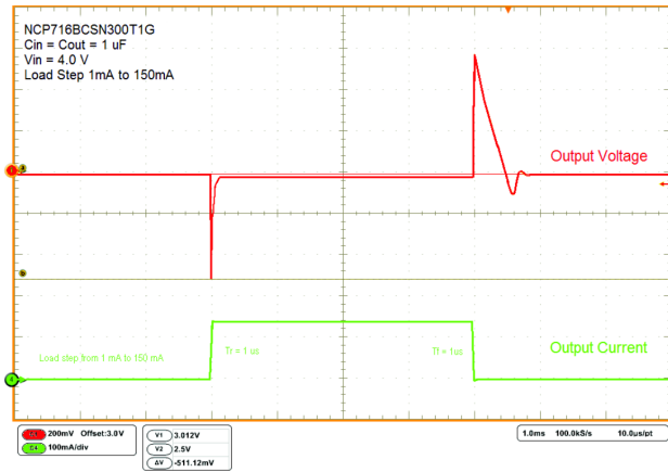
Figure 17. Load Transient Response
