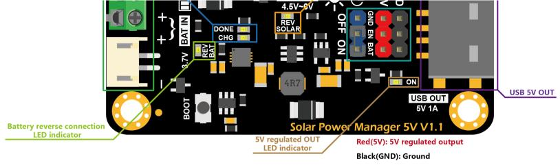
Blue(ON/OFF): 5V regulated output switch Use a jumper or a I/O pin to control the ON/OFF
