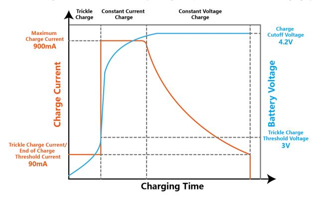
The module is designed for 5V (nominal/maximum power voltage) solar panel. Any kinds of panel (monocrystal, polycrystal, thin flim) can be employed as long as the **open circuit voltage** is less than 6.5V. Taking the size, weight, price of the panel and the 900mA maximum charge current of the module all these factors into consideration, it is recommended to connect a solar panel with no more than 10W to the SOLAR IN
