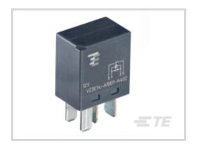
Rated Coil Voltage:12 VDCMicro Relay Contact Current Class:20 – 30 AMicro Relay Contact Arrangement:1 Form A (NO)Micro Relay Coil Resistance:119 ΩMounting Brackets:Without
