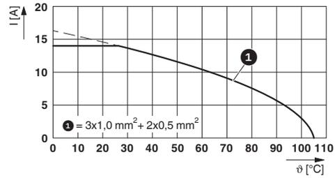
$I$  = current strength,  $\vartheta$  = ambient temperature, 3x 14 A + 2x 2 A constant
