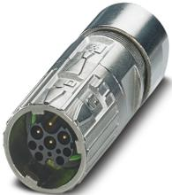
Cable connector, straight, shielded: yes, ONECLICK fast locking system, M17, No. of pos.: 5+3+PE, type of contact: Pin, Crimp connection, cable diameter range: 5.5 mm ... 9.5 mm, coding:N
