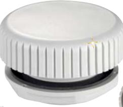
Installation: Make cut-out Ø 40.5 + 0.5 mm (1.6 + 0.02") in enclosure wall and mount pressure compensation device with nut. Please make sure that the sealing gasket is put in place on the outer side panel of the enclosure. For optimal pressure compensation we recommend to use two devices on opposite sides towards
