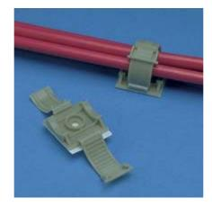
This clamp provides a fast and convenient method of securing bundles from .19" (4.8mm) up to .69" (17.5mm) diameter. It is available with adhesive backing or screw applied with one #6 (M3) screw.
