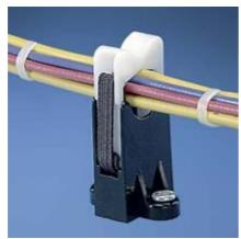
As wires are individually inserted, the bundle is pre-formed. When harness is complete it can be easily snapped out. Three sizes available for 1/2" (12.7mm) 3/4" (19.0mm) and 1 1/4" (31.7mm) bundles.
